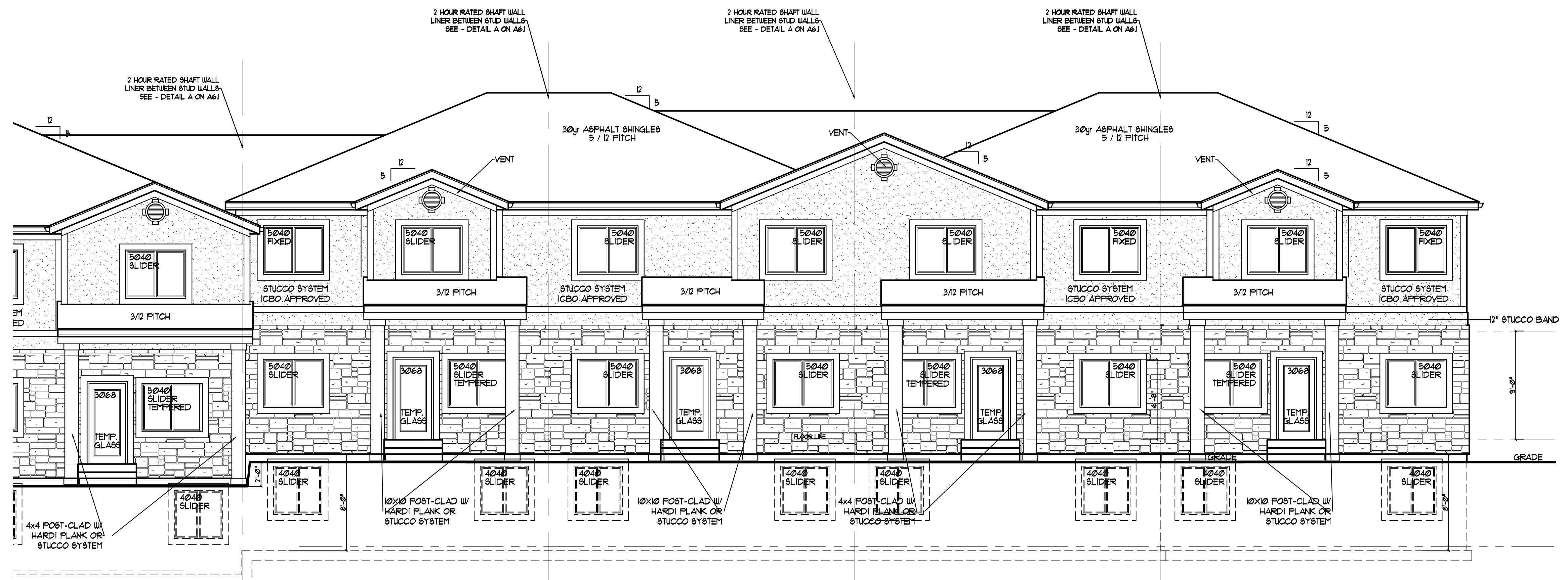
REAR ELEVATION scale - 3/16"=1'-0"
