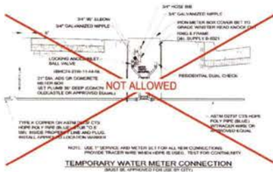
TEMPORARY WATER METER CONNECTION
